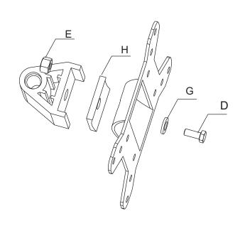
Fix the wall plat on the aluminium alloy joint with outer hexagond screw(D), iron washer(G), aluminium alloy insert(H) and screw nut(E).
