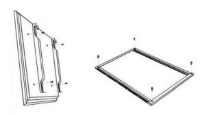
Thread the bolt through the appropriate washer, the arm and finally into the TV. Make sure the arms are vertically centered and level with each other.
